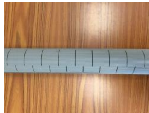
Old sub soil drain pipe Spacing: 3m apart
